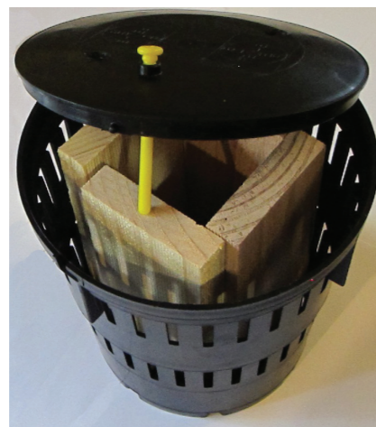
Larger timber sizes to increase time for active termite feeding.
